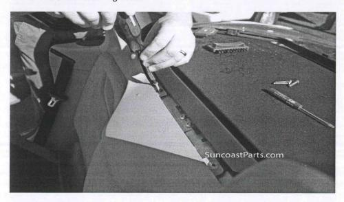
Gently pry apart the rollbar trim, just a small amount so you can insert the mounting guide:
