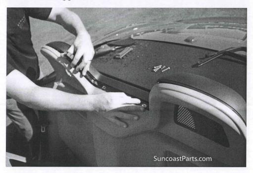
Tuck the upper portion of the guide behind the trim, make sure the upper button is flush with the trim when installed:
