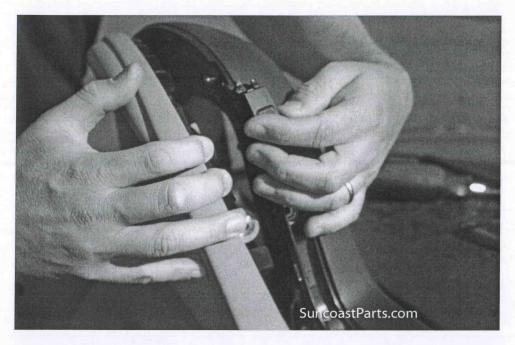
Once in place, squeeze the roll bar trims together. They should snap back into
